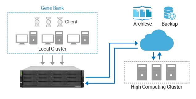
The EonStor GS and GSe Pro family of unified storage can accommodate both file-level (NAS) and block-level (SAN) applications from file sharing, e-learning, to digital library. Capacity can expand up to 1,792 drives or more than 20PB raw capacity. In addition, rich selection of connectivity options, form factors, and optional cloud storage gateway allow schools to meet the present and future needs.
